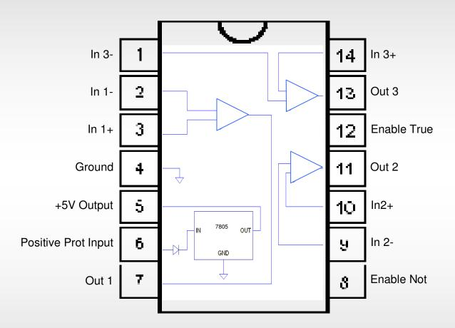
+5V voltage regulator and AM26LS32 line receiver IC, residing in a single package. The +5V regulator input is protected by a series diode.
